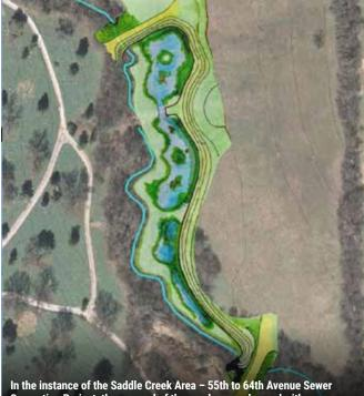
In the instance of the Saddle Creek Area – 55th to 64th Avenue Sewer Separation Project, the removal of the creek was enhanced with green infrastructure for stormwater retention.
